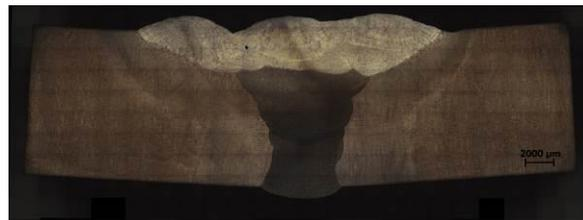
Fig.14 Micro structure of repair weld.
