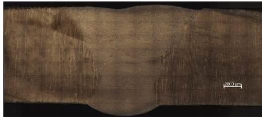
Fig. 12 Micro structure of Process II (Base metal, Annealing, Quenching, Tempering, Welding, Tempering(540°C)).
