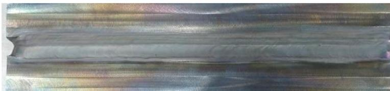
Fig. 8 Macroscopic surface of TIG welding.
